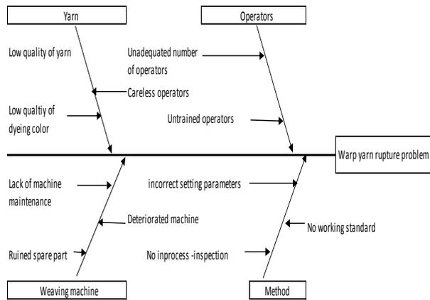
Fig. 4. The cause and effect diagram for warp yarn rupture problem
