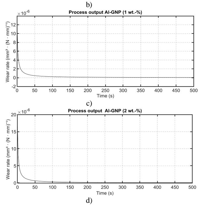
Fig. 4. Calculated wear rates: a) pure aluminum, b) 0,5 wt-% GNPs, c) 1 wt-% GNPs, d) 2 wt-% GNPs
