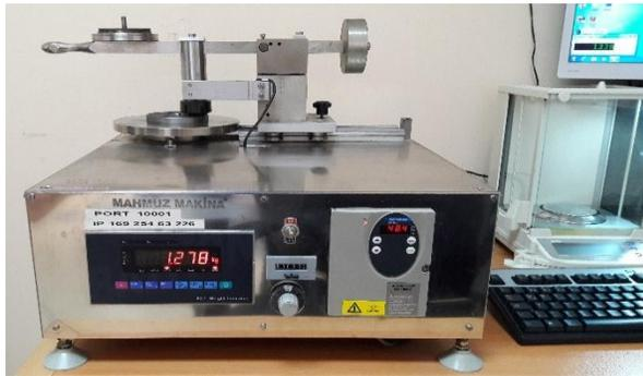
Fig. 1. Pin on disk experimental setup
