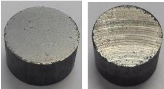
Fig. 2. Test samples of pin, before and after test.
