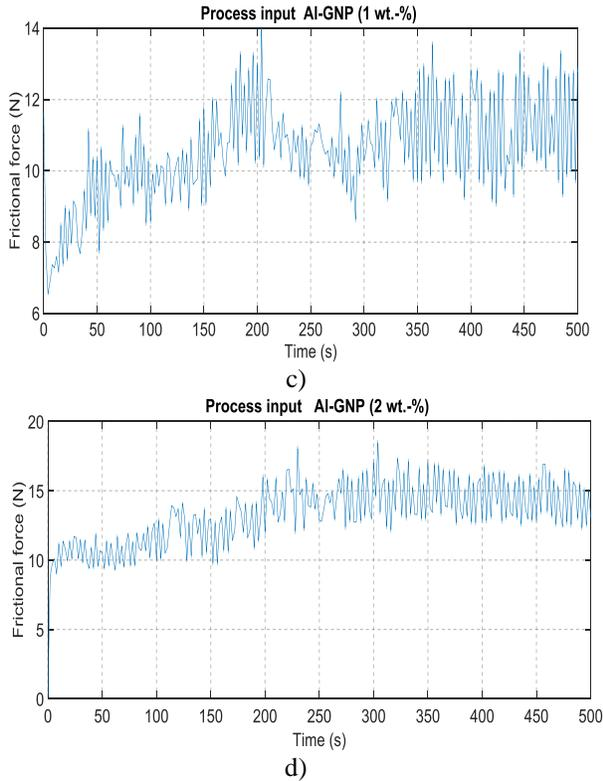
Fig. 3. Recorded frictional forces: a) pure aluminum, b) 0,5 wt-% GNPs, c) 1 wt-% GNPs, d) 2 wt-% GNPs
